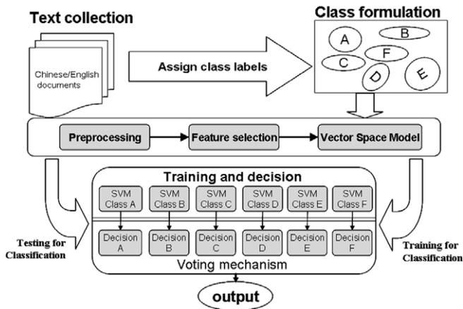
Fig. 6. System and process of the SVM-based MTC model.
