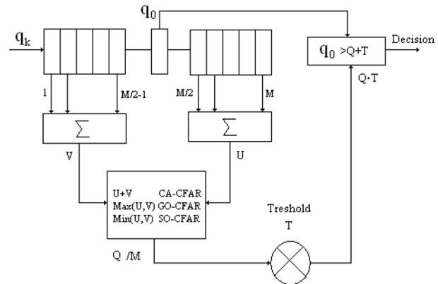
Figure 1. CFAR processor
