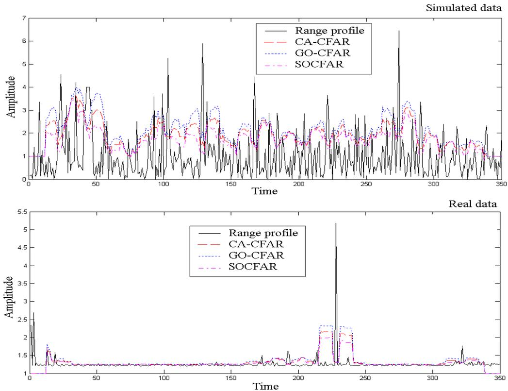
Figure 5 CFAR processor outputs
