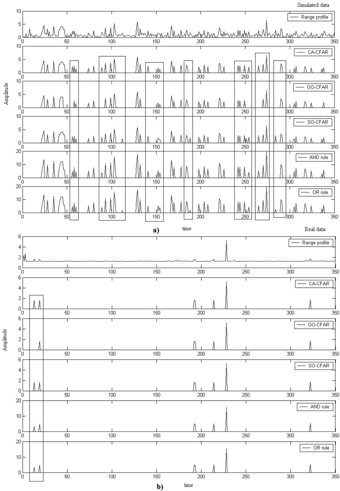
Figure 7 Target detections with fusion center
