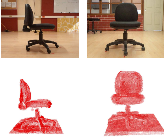
Fig. 10. Qualitative comparison of two views of the reconstructed object versus the real object. Almost all surface was seen, except the low part of the seat where the robot cannot reach due to the size of the arm.
