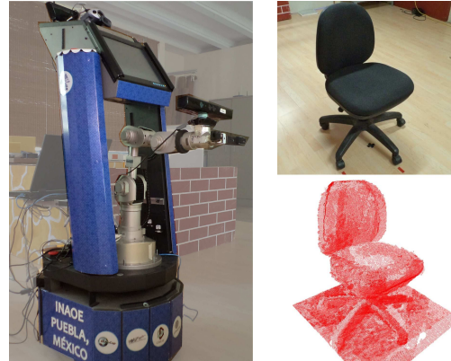
Fig. 1. The proposed method is able to plan each robot configuration in order to reconstruct a real object. In our experiments we use a mobile manipulator of 8 degrees of freedom to reconstruct a chair. A Kinect sensor was mounted on the robot’s end effector.
