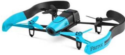
Fig. 7 Bebop quadrotor with bumpers.
