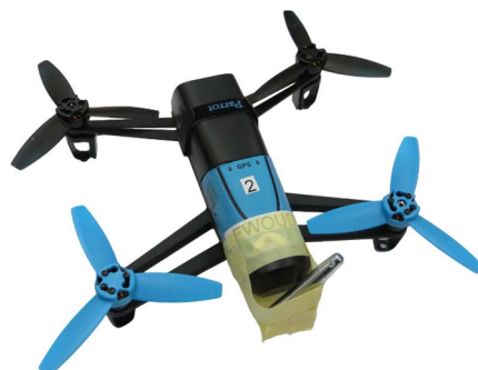
Fig. 6 Container attached to the nose of the quadrotor with one weight inside.
