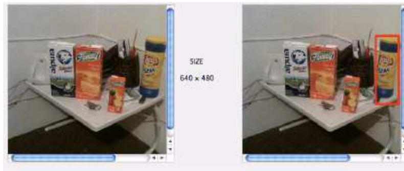
Fig. 6. Object recognition using measures of similarity. The object in the red rectangle is recognized in the image.
