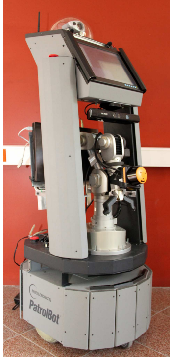
Fig. 1. Sabina , INAOE's service robot based on a PatrolBot platform
