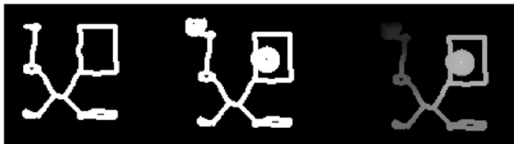
Fig. 13. Using the roadmap for navigation. From left to right: (a) Roadmap with an uncertainty of 20 cm. in the position of the robot. (b) The cells of the roadmap and the cells that connect the initial and final cells. (c) Values of V given by the value iteration algorithm (dark pixels denote high values)
