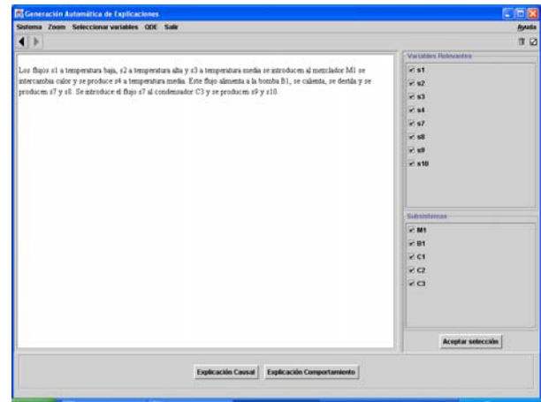
Figure 9 Functional explanation considering behaviors. The first sentence says: The flows s1 at low temperature, s2 at high temperature and s3 at medium temperature are introduced into the mixer M1 there is a heat exchange and s4 is produced at medium temperature
