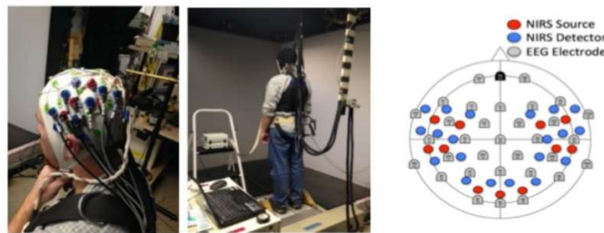
Figure 1. Concurrent NIRS-EEG was collected while standing for balance tasks.
