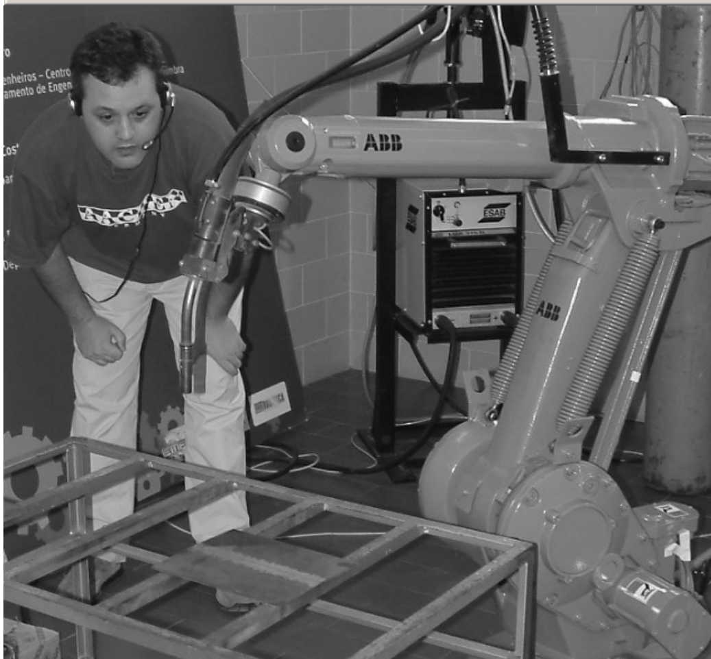
Figure 6: Shell of the voice interface application showing the welding operation, and a user (author of this paper) commanding the robot using a headset microphone.
