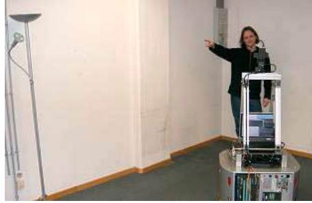
Fig. 1. Interaction with the mobile robot. Software components of the robot include: speech recognition, speech synthesis, person and gesture tracking, dialogue management and multimodal fusion of speech and gestures
