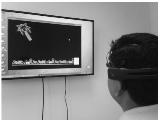
Fig. 3. Headset and stimulus used for the experiment on P300 signal detection.
