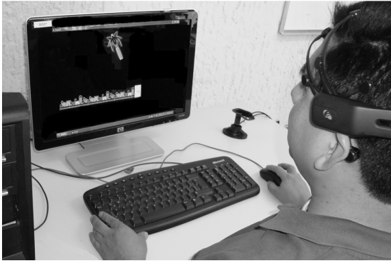
Figure -3. Headset and stimulus used for the experiment on P300 signal detection.
