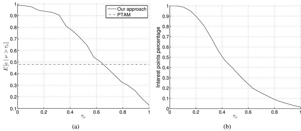
Fig. 6. Our model as an alternative to PTAM initialization. (a) Empirical estimate of the expected value of the fractional error conditioned to the estimated confidence  $\hat{\nu}_i$  is greater than a given threshold  $\tau_\nu$ . (b) Percentage of interest points for which  $\hat{\nu}_i > \tau_\nu$  as a function of  $\tau_\nu$ .
