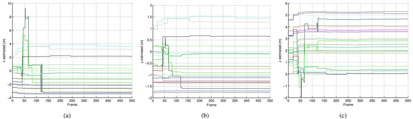
Fig. 7. Spatial-temporal evolution of interest points possessing high confidences. Evolution over time of the 3-D coordinates of the reconstructed landmarks with highest confidences, after a typical initialization. Each curve corresponds to a specific point initially introduced to the map using our method. (a)  $x$ -coordinate. (b)  $y$ -coordinate. (c)  $z$ -coordinate.
