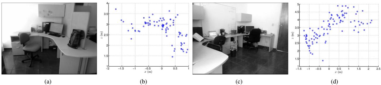
Fig. 8. Initial map, made of high confidence interest points. Note that the scene structure is captured by the point cloud. (a, c) Acquired image. (b, d) Scene map, viewed from a top perspective.
