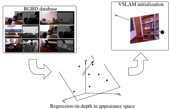
Fig. 1. Overview of our system: We use collected RGB-D data (upper left part) to learn regression parameters in an appearance space (lower part) around corner points to infer depth. The inference system is used to initialize a VSLAM system from a single shot (upper right part).
