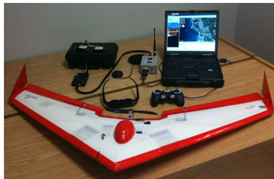
Fig. 5. Our robotic platform is a commercial fixed-wing UAV with an on-board autopilot microprocessor and a gimbal-mounted camera.
