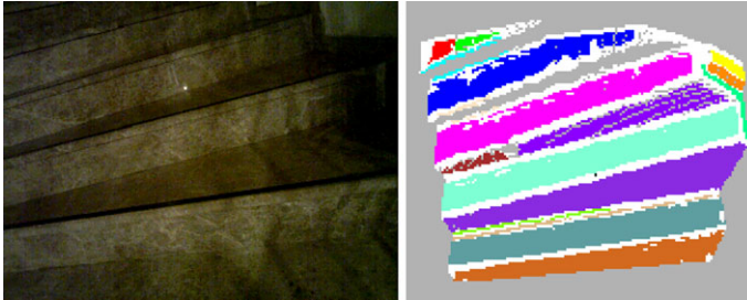
Fig. 9 One image of spiral stairs and its point cloud segmentation result
