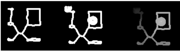
Figure 17: Using the roadmap for navigation. From left to right: (a) Roadmap with an uncertainty of 20 cm. in the position of the robot. (b) The cells of the roadmap and the cells that connect the initial and final cells. (c) Values of V given by the value iteration algorithm (dark pixels denote high values).
