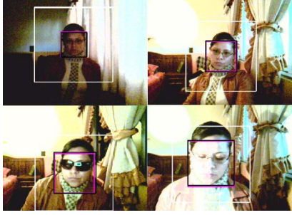
Figure 1. Examples of the performance of the tracking algorithm under different conditions. In each image, the inner rectangle corresponds to the Viola–Jones face detector; and the outer rectangle to the search window.
