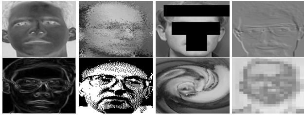
Figure 6. Sample image with the following effects (from left to right)negative, oil paint, cutting regions, emboss, edge detection, decreasing color depth, twirl and pixelizing
