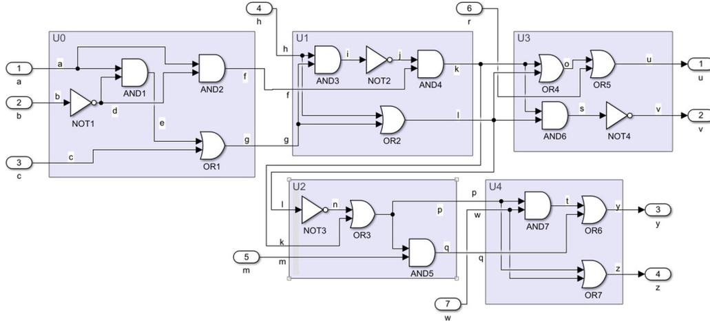
**Fig. 3.** Combinational logic circuit partitioned into 5 components.
