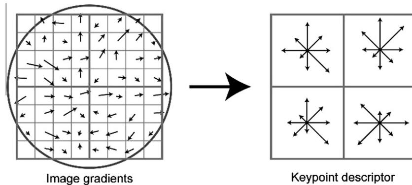
**Fig. 5.** This figure, for purposes of explanation, shows a descriptor of  $2 \times 2$  regions calculated from a region of  $8 \times 8$  pixels, but Lowe proposes to use descriptors of  $4 \times 4$  regions in neighborhood of  $16 \times 16$  pixels around the point.
