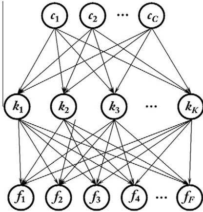
**Fig. 3.** Graphical representation of the three layer Bayesian network used to classify a new object. In the first layer we have the classes for which the model was trained. The nodes in the second layer represent the clusters obtained in the training phase. Finally, the third layer represents the features extracted from the new object.
