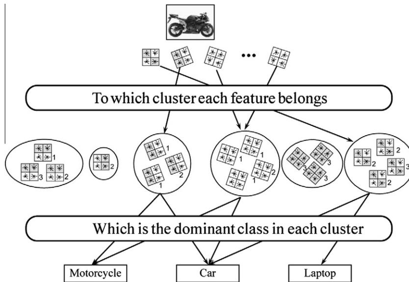
**Fig. 2.** Classification scheme for a new image. SIFT features are extracted from this image and for each feature the cluster from the learned model to which it belongs is identified. The object class is the majority class in these clusters.
