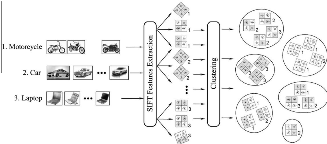
**Fig. 1.** SIFT local features are extracted from the training set formed by several sample images per class. Later, features descriptors are clustered (the elements inside each circle represents a cluster). Each feature in each cluster is labeled with its corresponding class (represented in the figure by the subscripted number on every element of a cluster). Note that features from different classes could be in the same cluster.
