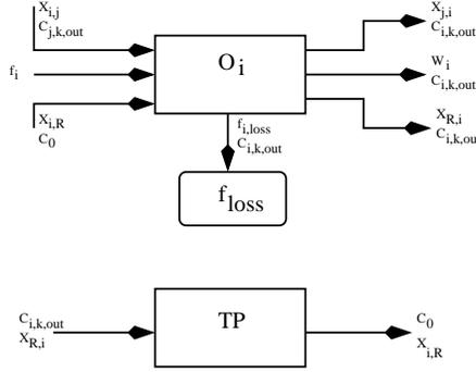
**Fig. 2.** General structure for mass balance.
