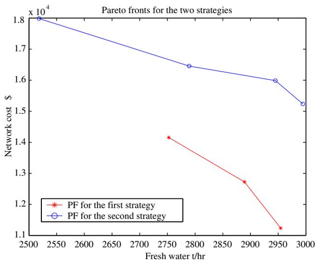
Fig. 14. Comparison of the Pareto fronts obtained for the two strategies used for the Cuernavaca city water distribution system.
