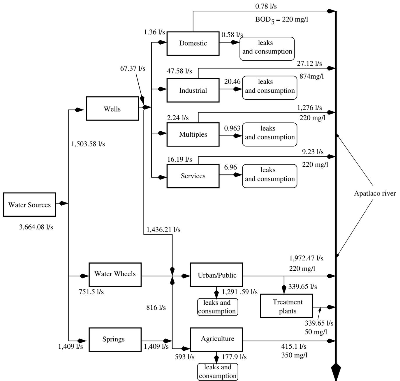
Fig. 10. Current operation of the distribution system of the city of Cuernavaca, Mexico.
