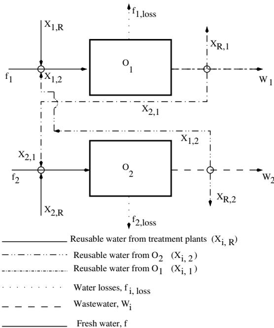
Fig. 1. Block diagram of a water-using system with two sources and two operations.
