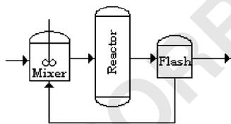
Fig. 18. MRF system, a cyclic physical device with three components.
