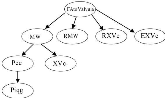
Fig. 4. Network obtained automatically by applying the K2 algorithm for fuel valve fault.
