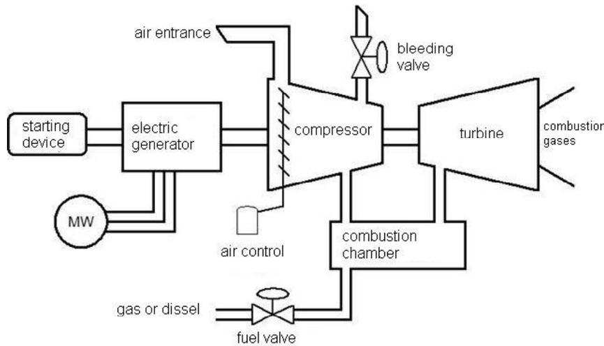
Fig. 3. Simplified schema of a gas turbine.
