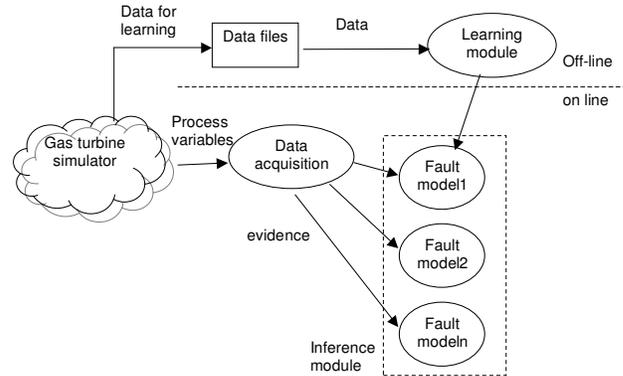
Fig. 2. Proposed software architecture for multiple faults diagnosis of gas turbines.
