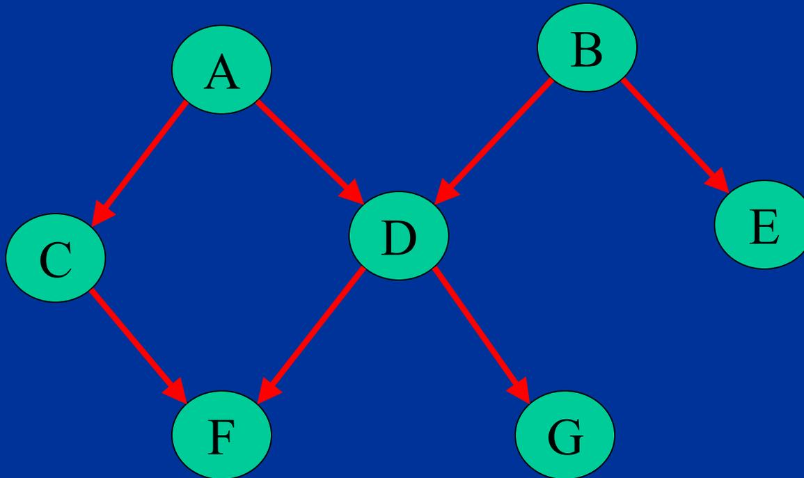
$$\begin{aligned} & P(A,B,C,D,E,F,G) \\ = & P(G|F,E,D,C,B,A) P(F|E,D,C,B,A) P(E|D,C,B,A) \\ & P(D|C,B,A) P(C|B,A) P(B|A) P(A) \\ = & P(G|D) P(F|D,C) P(E|B) P(D|B,A) P(C|A) P(B) P(A) \end{aligned}$$
