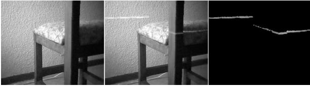
Figure 5: Laser range sensor operation. From left to right: (a) Image from the camera. (b) Image with the laser line generator turned on. (c) Image of (b) - (a)
