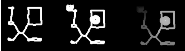
Figure 7: Using the roadmap for navigation. From left to right: (a) Roadmap with an uncertainty of 20 cm. in the position of the robot. (b) The cells of the roadmap and the cells that connect the initial and final cells. (c) Values of V given by the value iteration algorithm (dark pixels denote high values)
